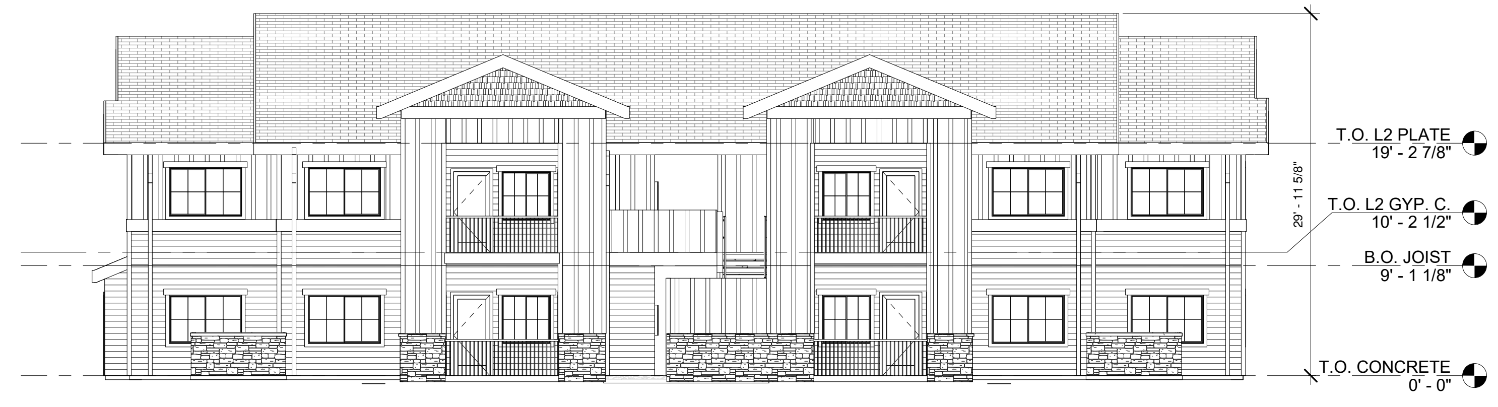
④ REAR ELEVATION - BLDG. TYPE B 1/8" = 1'-0"
