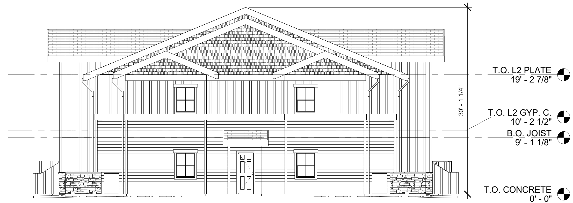
3 RIGHT ELEVATION - BLDG. TYPE A 1/8" = 1'-0"
