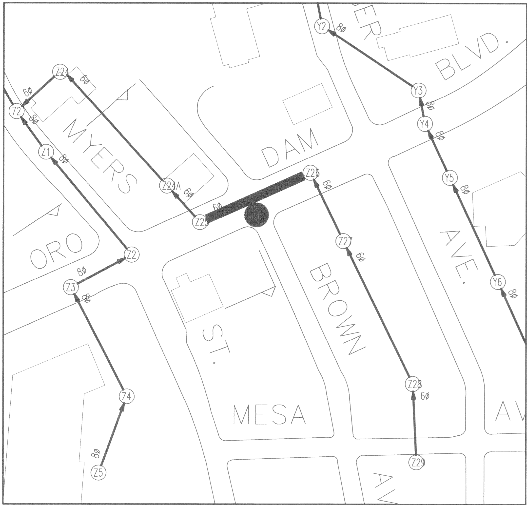
6" TERRA COTTA PIPE ALONG ORO DAM BOULEVARD
