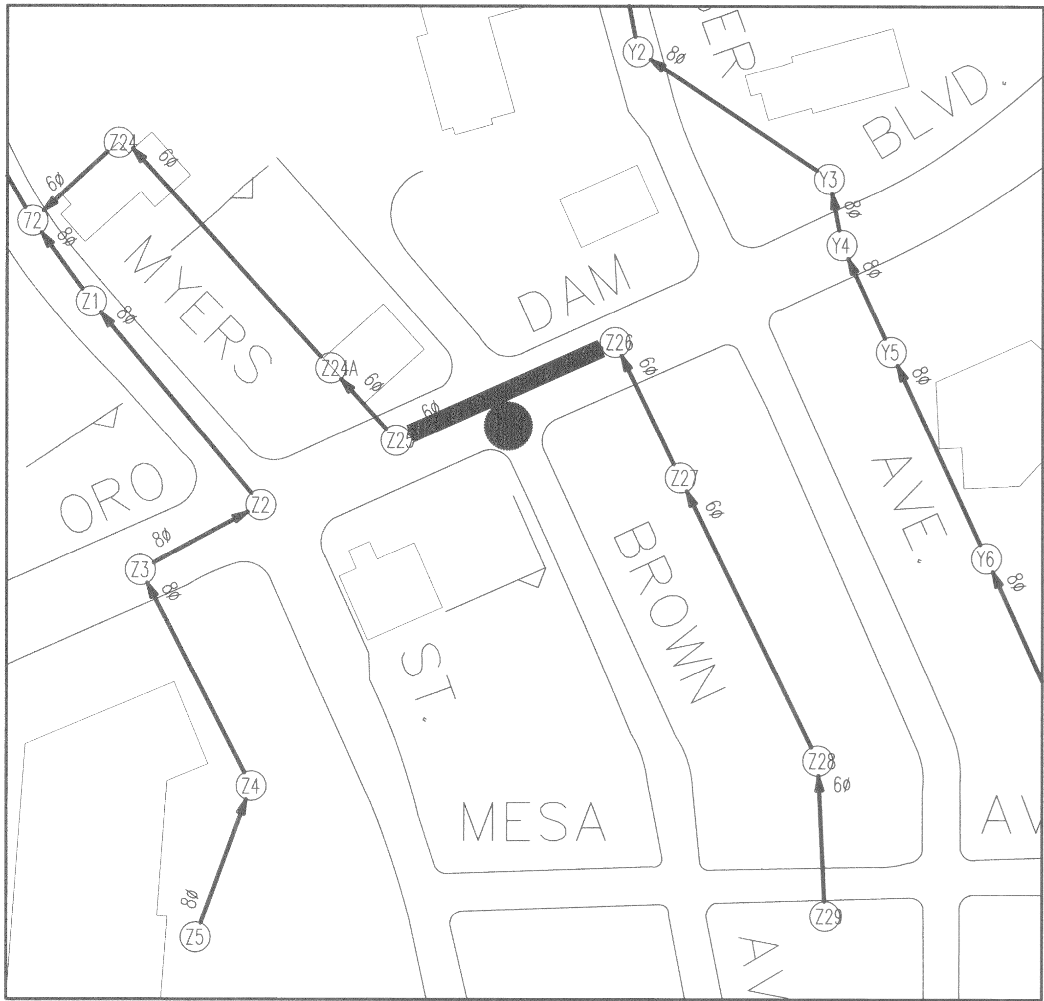
6" TERRA COTTA PIPE ALONG ORO DAM BOULEVARD
