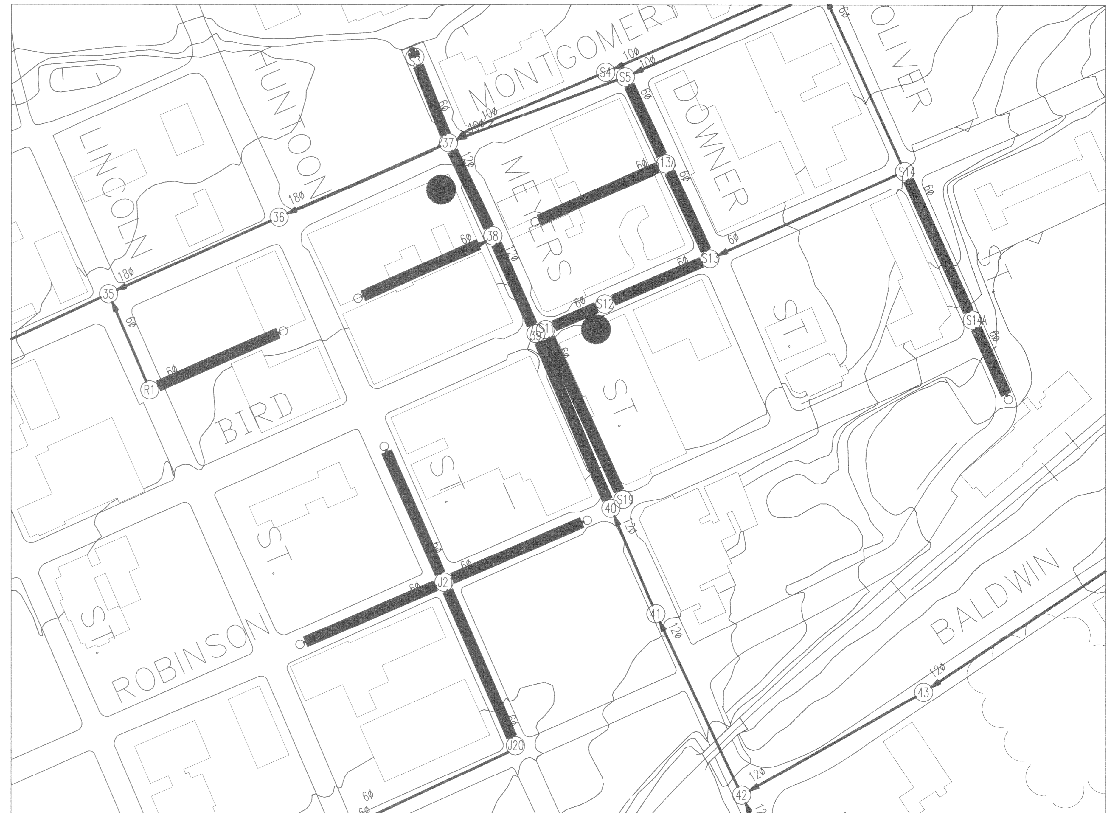
6" - TERRA COTTA PIPE ALONG: MINERS ALLEY, HUNTOON, ROBINSON, MEYERS, BIRD, AND OLIVER STREETS
