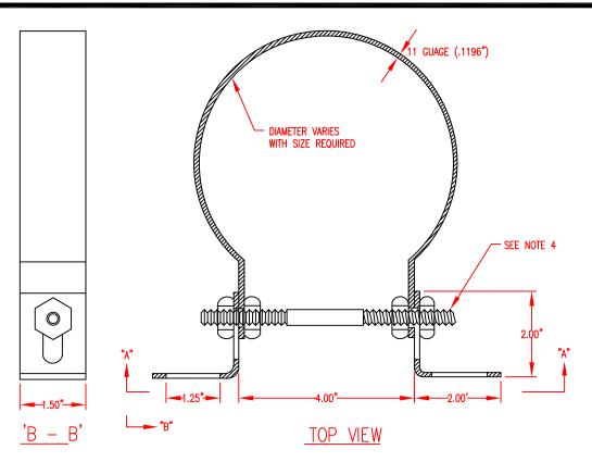
STAINLESS STEEL ADJUSTABLE CLAMPING BRACKET AS MANUFACTURED BY RELINER-DURAN, INC. OR APPROVED EQUAL.
